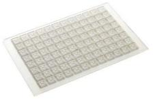
Designed to reduce evaporation when cycling 96-well plates.
