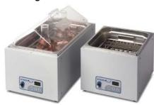
Linear shaking water baths with stainless steel tank and simple, intuitive 3 button user interface. It is quick and easy to fit alterative shaking trays. Heating element is positioned on the underside of tank, no heating element in the bath means it is easier to clean and keep clean. Baths have an independent sample protection feature. Available ready to use in two sizes to suit a variety of applications including sample preparation, mixing and thawing.
