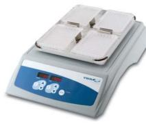
Microplate shakers with microprocessor control which hold two or four microplates, deep well plates or two microtube racks. Variable speed across a wide range may be adjusted to suit the application; a low speed ensures that the well contents are not ejected, more vigorous agitation provides effective aeration across the small surface area of each of the wells. Ideal for use in immunology, biotechnology, microbiology and pharmacology applications.
