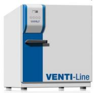
Drying ovens with forced air circulation, which are ideal for routine drying and heating applications when short drying times are required. Ovens feature adjustable ventilation by means of manually adjustable ventilation slide and 50 mm Ø exhaust duct at the rear of the unit.
