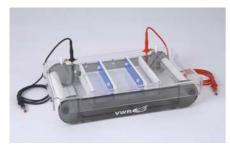
The kuroGEL Midi Plus 15 Horizontal standard gel electrophoresis unit provides the most popular comb throughput and tray-size options, but with additional casting options.
