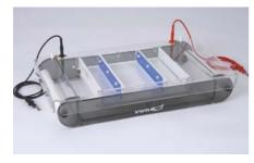
The kuroGEL Maxi 20 Horizontal gel electrophoresis unit is ideal for high resolution analytical and preparative studies of nucleic acids. Large format, 20×20 cm, gel tray is ideal for high resolution techniques, such as screening PCR products and RFLP analysis.
