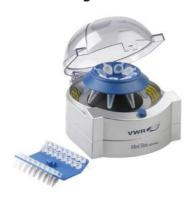
This centrifuge was developed for applications that do not require high speed centrifugation, such as micro-filtration and cell separation, and can also be used in a cold room. Metal base with ABS body and transparent safety cover. On closing the lid, the rotor quickly accelerates to maximum speed. Pressing the button on the front of the unit stops operation and opens the lid. Alternatively, the unit can be turned on and off with the switch on the back.
