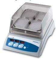
Incubating microplate shaker with microprocessor control which hold four microplates or two microtube racks. The speed can be adjusted across a wide range to suit the application; a low speed ensures that the well contents are not ejected, more vigorous agitation provides effective aeration across the small surface area of each of the wells. Ideal for use in immunoassays, hybridisations, biotechnology, microbiology and pharmacology applications.
