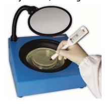
The viewer for colony counting has a plexiglas rest surface with cm graduation scale, cold-light indirect fluorescent lighting and magnifying glass adjustable for correct positioning. Counting pen not included.
