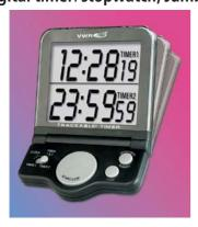
This timer allows simultaneous programming of two different activities from 24 hours to 1 second. Each channel has a distinct electronic alarm and display indicator when zero is reached. The alarm may be turned off or it is silenced automatically after 1 minute. A second display mode shows time of day and a stopwatch (for count-up timing).
