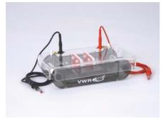
The kuroGEL Mini 6 Horizontal is ideal for routine preparatory and analytical electrophoresis techniques.
