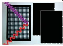
These films are 200  $\mu$ m thick black vinyl with adhesive for use with 96-well, 384-well, and 1536-well black microplates. They fit within the edges of raised-rim plates and may be applied to either the plate top or bottom. The light-blocking and absorbing properties of these films make them ideal for reducing stray light and crosstalk in fluorescence applications and for protecting light-sensitive samples in storage.
