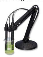
Electrode arm moves smoothly in almost any direction, holding up to 4 electrodes + 1 temperature sensor safely and securely in selected positions. Fingertip control raises, lowers, and pivots the holder. The arm articulates at three points while maintaining electrodes in a vertical position.
