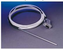
Remote temperature probes for use with circulators with a programmable controller. Permit points of control to be switched from inside a programmable circulator bath to a remote location, such as an open tank. Compensates for heat loss through tubing between the circulator and the control point. Platinum RTD sensor with stainless steel sheath. Rubber coupling with 25,4 mm Ø, connects sheath to flexible cable. Probe cable ends in a DB9 female plug.
