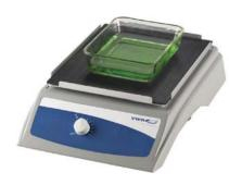
General purpose shaker with microprocessor control which is ideal for basic mixing applications, blotting techniques, staining and destaining. Variable speed control provides consistent, uniform shaking action. The speed is adjustable via knob with 1 to 10 dial settings and the ramping feature slowly increases speed to the set point for added safety.
