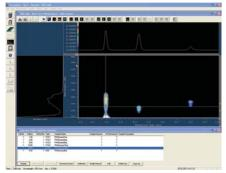
Chromatography Data System (CDS) for control of the VWR Hitachi Chromaster™ 400 bar system only.
