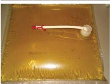
The T bag is filled with pre-weighed granulated media. Connect the filter unit,  $0.2 \mu m$ , aseptically to the tube by using the the connector device. Add sterile water under aseptic conditions into the bag via the filter sytem. Protect the tube end with the red cap.
