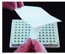
These films are 200 µm thick white vinyl with adhesive, for use with white microplates. Light reflective properties of the film, when used to seal clear-bottom plates, maximise the sensitivity of bioluminescence and chemiluminescence assays in bottom-reading luminometers. White films have also been used as a backing matrix for microscopy of punch-out samples from filter plates.
