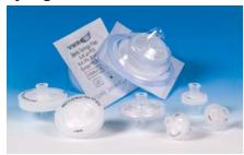
Membranes with pore size of 0,2  $\mu$ m are used for filtration of fine particles, those of 0,45  $\mu$ m are appropriate for clarifications.
