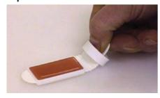
Dip slides for semi-quantitative monitoring of surfaces and in liquids. Testing with dip slides is a safe, reliable, economical and fast indicator of the presence of microorganisms. The dip slides with a push cap have a larger contact area.
