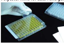
These 50 µm thick polyester films provide secure sealing around every well, not just a cover, thus minimising evaporation, preventing spillage and well-to-well contamination, and eliminating "edge effects" in sensitive ELISA assays. Polyester films can also be used with tissue culture plates for short-term storage, incubation, and containment of biohazards.
