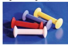
PTFE covered, strong Alnico V magnetic core. Smooth surface. Very good centring, small footprint and high turbulence even at low speeds. Disc diameter 20 mm, rod diameter 8 mm.
