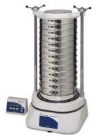
The three electromagnetically driven test sieve shakers are designed for sieve analysis with optimum three-dimensional sieving action. The self re-adjusting amplitude, which uses permanent acceleration measurement of the whole sieve tower, balances the oscillation of the shaker and its stand. This guarantees that amplitude stays the same, irrespective of the feed quantity and the installation position.
