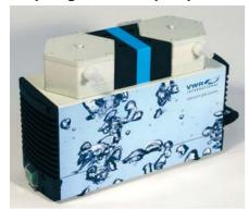
Dual-head, dry running diaphragm pumps for a wide range of laboratory applications. They pump, compress and evacuate without affecting media, i.e. media remains uncontaminated. The pump includes a diaphragm with patented tension optimisation, which allows the pump to be smaller and prolongs the service life of the diaphragm.
