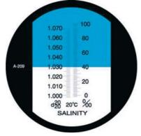
These robust refractometers are easy to use and deliver exact, consistent results. There are several different models with the relevant scale (°Brix, specific gravity, Oechsle) for juices, beverages, industrial liquids, etc.
