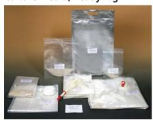
Each bag contains a pre-weighed amount of granulated media in a double bagged bag and is irradiated. Just in time enrichment - add sterile water and sample material.
