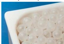
Lightweight, economic PP spheres which form a blanket on the liquid surface. Spheres have 20 mm Ø, 275 spheres cover approximately 1000 cm<sup>2</sup>.
