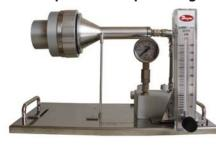
Pinocchio Super II is a microbial impaction sampler to test the microbiological quality of compressed air and gases used in cleanroom. A compressed air source is connected to the Pinocchio Super II system and the flow meter regulated to achieve the required flow rate, e.g.: 100 litres of air / minute. The sampling period is timed to obtain the required total sample volume, e.g. 1000 litres.
