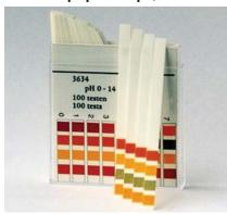
The test strips contain indicator dyes that are covalently bound to the reagent papers and then adhered to plastic strips. Contamination of the solution is therefore prevented even in strong alkaline solutions or from long immersion in weak buffered solution.
