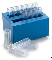
Two parallel slots fit 6 cuvettes in each slot, side by side for excellent stability and heat transfer.
