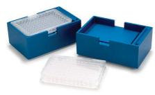
Recessed well for better stability; flat surface is good for flat and round bottom plates. Fits 2/4/6 block heaters.
