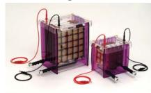
VWR Collection electroblotting unit is designed to provide a safe and easy to operate system for the transfer of nucleic acid or proteins from a gel matrix onto a suitable transfer membrane. It can be used to blot up to four gels of 10×10 cm.
