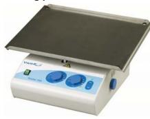
Rocking platform shakers have variable speed and adjustable tilt to provide optimum control of mixing conditions, a gentle wave motion is ideal for blotting membranes and gels. Shakers maintain constant speed regardless of load or voltage fluctuations. Durable shakers with choice of models with single- or double-tiered stainless steel platforms.
