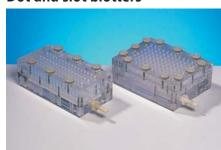
Machined from high density acrylic with precision lapped mating surfaces to ensure uniform filter contact, these manifolds are designed for DNA and RNA membrane hybridisations and antigen/antibody screening in immunological applications. Each manifold consists of paired upper dot- or slot-forming modules and a lower vacuum chamber module. A vacuum of approximately 600 mm Hg (0.8 bar) is required during sample application.
