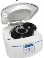
Safe and easy to use centrifuge delivering optimum performance in a compact unit. All operating parameters, including rpm, RCF and remaining time, are set and displayed digitally. It has an automatic door release, pulse spin function for fast, convenient quick spins and an unique internal airflow design to reduce the heating up of samples.
