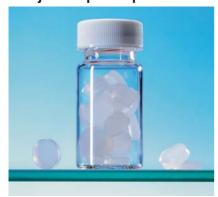
Long-life GC-septa for inlet temperature of up to 340 °C.
