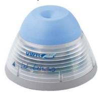
Vortex mixer suitable for single small containers up to 30 mm in diameter, for example test tubes, centrifuge tubes and microtubes. The upper casing is PP and the test tube surface is made from inert TPU plastic; the bottom section is a coated, zinc die-casting.
