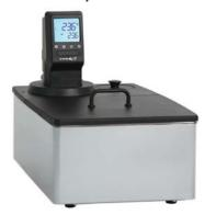
Stainless steel baths with user friendly MX temperature controller with three control buttons and on-screen prompts. The convenient slide control enables the flow rate to be easily adjusted. Baths can be used for external circulation, the controller bridge made from chemically resistant DuraTop™ is easily removed to clean the tank. The 10 and 20 litre models have an opening with lid for optional cooling coil which is ideal for set points near ambient temperature.
