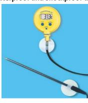
Stainless steel probe (Lר: 127×3,6 mm) with three metre cable
