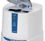
The PCR Plate Spinner offers a personal sized centrifuge designed to spin down PCR plates. This unique centrifuge is equipped with a dual position vertical rotor that accepts a wide variety of PCR plates; 96-well, 384-well, skirted and non skirted plates are compatible with the Plate Spinner. The rotor features integral plate guides, ensuring that the plates stay vertical and do not tip inside the rotor.
