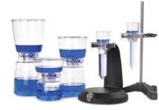
Designed for the preparation of buffers, tissue culture media, microbiological media and other biological fluids. These vacuum filtration systems feature large diameter Pall membranes for guaranteed performance and maximum throughput. The bottle-top filtration system design includes a receiver bottle with an ergonomic shape, moulded finger grips and a patented bottle cap. The centrifuge tube and funnel system, allows the user to filter fluids directly into a 15 ml or 50 ml tube.
