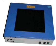
All GenoView transilluminators have variable intensity settings and even illumination. A 302 nm transilluminator is supplied as standard with each GenoPlex system.
