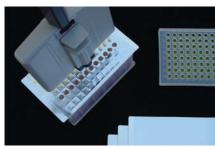
These soft non permeable  $38~\mu m$  thick aluminium foils with strong medical grade adhesive eliminate the need for heat-sealing devices or mats during thermal cycling. Compared to other aluminium foils, these foils have less tendency to roll back on themselves when removing the backing paper and fit well to the plate during application. Sterile product is packaged in tamper evident bags of 25/bag.
