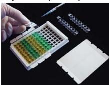
Polyester 2×8 strip films are identical to polyester films in material and adhesive, but designed for sealing only one or two 8-well rows at a time on either strip-well plates or standard plates whenever rows must be selectively protected or accessed. Sterile product is packaged in tamper evident bags of 50/bag.
