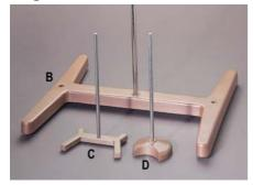
H-shaped stands with nickel-coated steel rod and 420×400 mm grey marbled cast iron baseplate.
