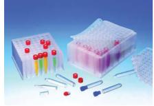
96-Position systems (Ritter) with glass inserts are used in HTS (high throughput screening) chemistry when the pure PP block is not inert enough. The inserts can be sealed with a PE cap seal or over the whole block with a Sealmat block cover made of silicone laminated with a PTFE film.
