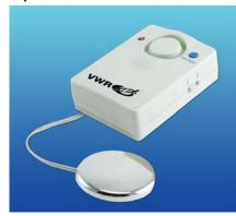
It can be used to detect when drums, tanks, flasks, or beakers are close to overfilling. The moment a solution touches the sensor, the alarm sounds and a red light flashes continually until the liquid no longer touches the sensor.
