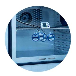
Mapping with different temperature probes (from 1 to 9 points) with variable time. (between 1 hour and 24 hours)
